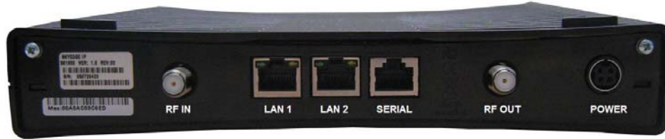
Figure 9: SkyEdge II Extend VSAT - Rear view with Connections Labeled
