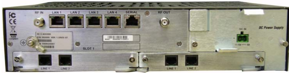
Figure 6: SkyEdge II Access VSAT - Rear view with Two FXS Add Ons and DC Power Supply
